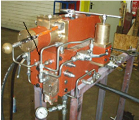
offshore valve block overhaul
